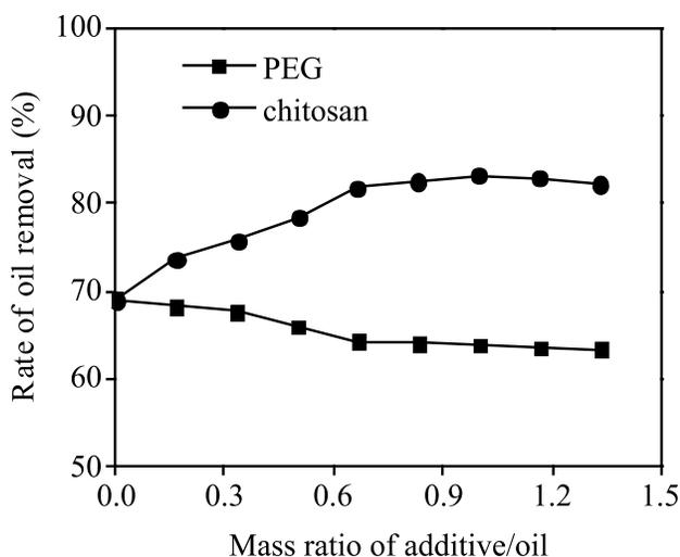
**Fig. 6.** Additive concentration in the wastewater as a function of the rate of oil removal. The reactions were conducted for 6 h with an initial oil concentration of 120mg/L, laccase concentration of 3 U/mL, pH of 6.0, and temperature of 30°C.
