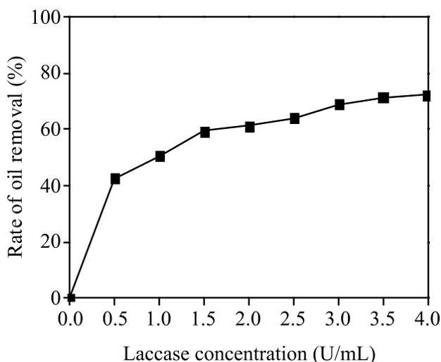
**Fig. 2.** Effect of laccase concentration on the rate of oil removal. The reactions were conducted for 6 h with an initial oil concentration of 120mg/L, pH of 6.0, and temperature of 30°C.
