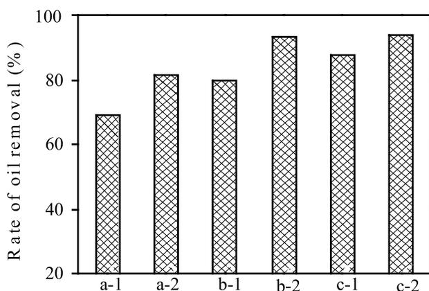
**Fig. 7.** Effect of water component on the rate of oil removal. The reactions were conducted for a reaction time 6 h with initial oil concentration of 120 mg/L, laccase concentration of 3 U/mL, pH of 6.0, and temperature of 30°C. a-1 = synthetic water; a-2 = synthetic water + 80mg/L chitosan; b-1 = polluted water; b-2 = polluted water + 80 mg/L; c-1 = circulating water; c-2 = circulating water + 80mg/L chitosan.
