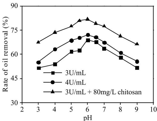
**Fig. 1.** Effect of pH on the rate of oil removal. The reactions were conducted for 6 h with an initial oil concentration of 120mg/L and temperature of 30°C.
