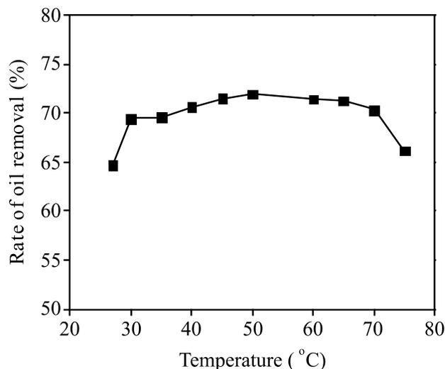
**Fig. 3.** Effect of temperature on the rate of oil removal. The reactions were conducted for 6 h with an initial oil concentration of 120mg/L, laccase concentration of 3 U/mL, and pH of 6.0.
