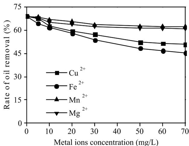
**Fig. 5.** Effect of metal ions on the rate of oil removal. The reactions were conducted for 6h with the initial oil concentration of 120mg/L, laccase concentration of 3U/mL, pH 6.0, and temperature of 30°C.
