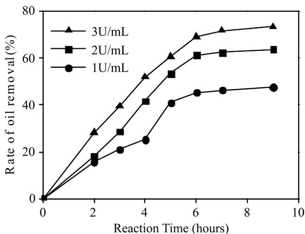
**Fig. 4.** Effect of reaction time on the rate of oil removal. The reactions were conducted with the initial oil concentration of 120mg/L, laccase concentrations of 1, 2, and 3 U/mL, pH of 6.0, and temperature of 30°C.
