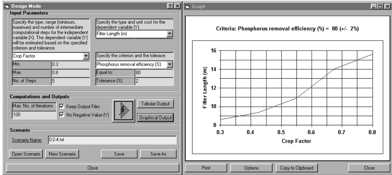
Fig. 3. Data preparation for the application of GDVFS in design mode.
