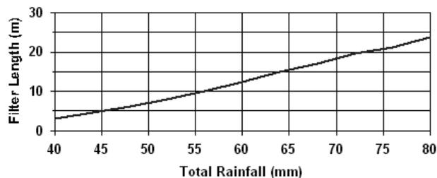
Fig. 4. Change in length of the VFS with rainfall depth obtained by the application of the GDVFS in design mode. Criteria: Sediment Removal Efficiency (%) = 80 (+/- 1%).
