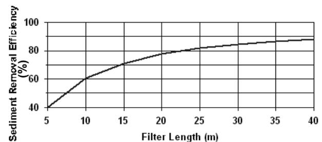
Fig. 5. Relationship between the length of the VFS and the sediment removal efficiency obtained by application of the GDVFS in design mode.
