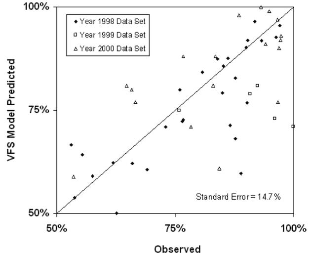
**Fig. 1.** Comparison of observed and simulated phosphorus removal efficiencies of the VFS.
